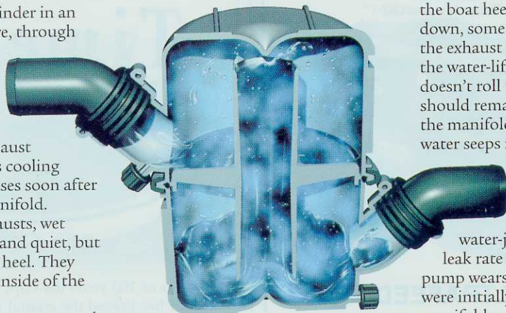
Modern water-lifts are light, corrosion-free, and often incorporate baffles
